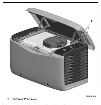
Figure 1-4 Removing the Air Intake Panel
